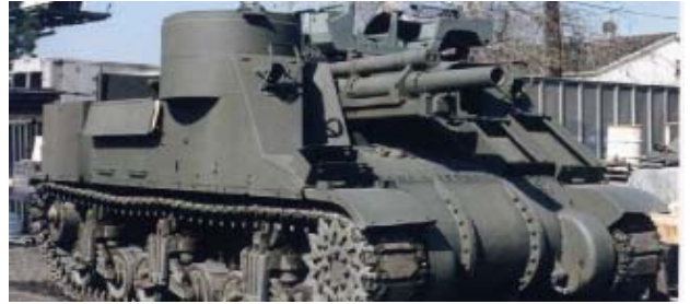
In the 1940s and 50s, the concept of “self-propelled” artillery took shape. Shown above is a 105mm M7 “Priest” self-propelled artillery piece.
